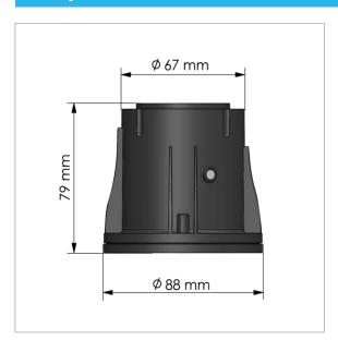
**U-Spot M2M** is a wireless parking sensor that measures, every 3 seconds (configurable), the Earth's magnetic field changes produced in a parking space.
